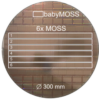
Fig. 2. Processed wafer with 6 numbered MOSS sensors in the centre, and one of the overall 23 babyMOSS sensors labelled near the top of the wafer.
