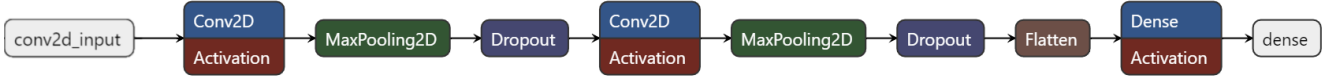
Figure 5. CNN architecture adopted for the experiments. Two 2D convolutional layers, followed by as many max-pooling layers, precede the dense layer and the two final neurons used for classification.
