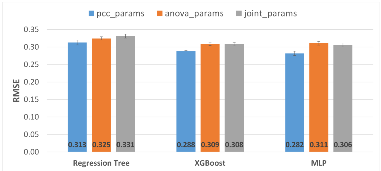
Figure 2.3: RMSE results achieved by the 3 regression models when trained on the 3 features datasets.
