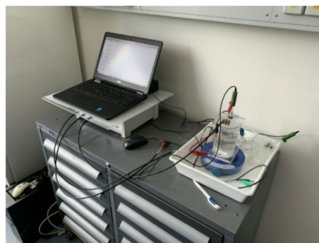
Fig. 2 (a) Experimental setup used for the potentiodynamic polarization tests; (b) of the electrochemical cell, highlighting the electrical connections between working, reference, and counter electrodes
