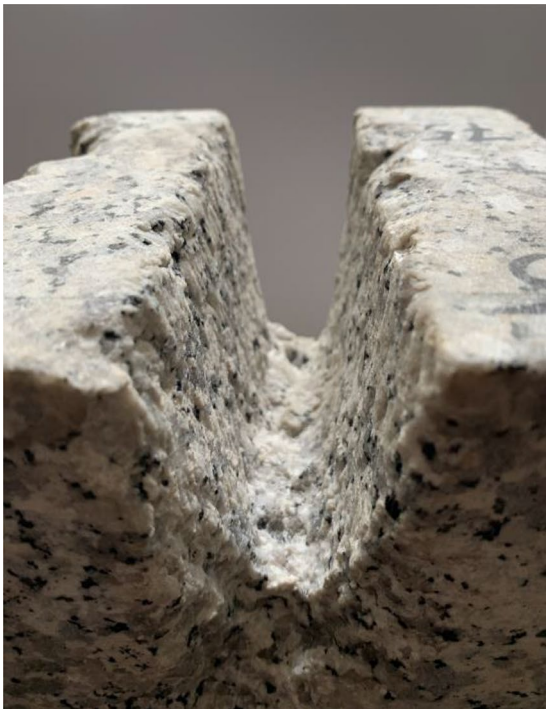
Fig. 7 Resulting grooves (about 5 cm wide) in loaded samples of Rosa Beta granite
