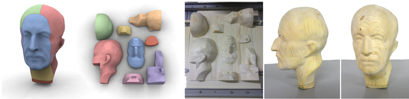
Fig. 1. We decompose general 3D geometries into height-field blocks (left), enabling their fabrication using single pass 3-axis CNC machining (right).
