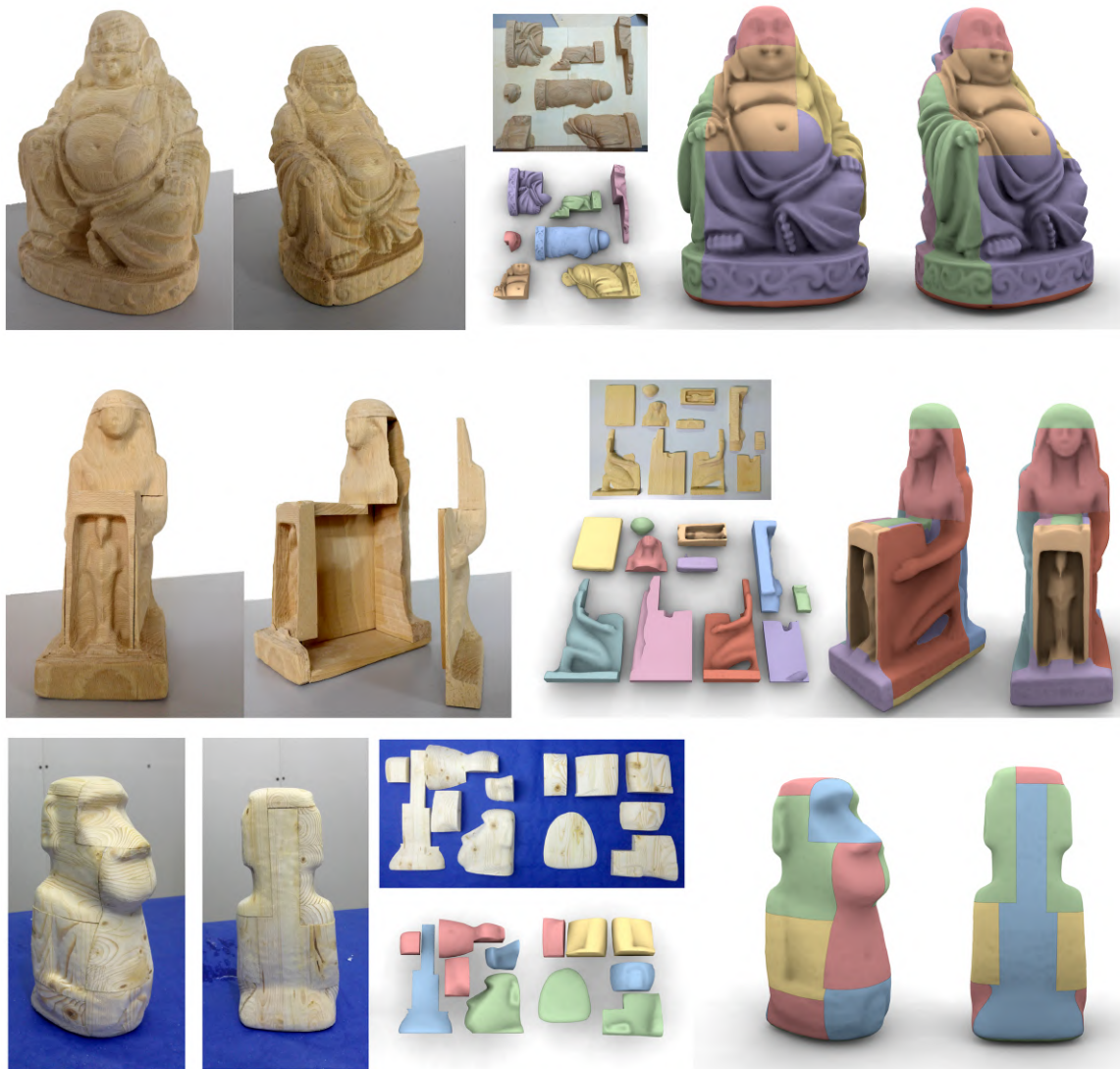
Fig. 12. A gallery of decompositions computed with our algorithm and fabricated in wood using a 3-axis milling machine.
