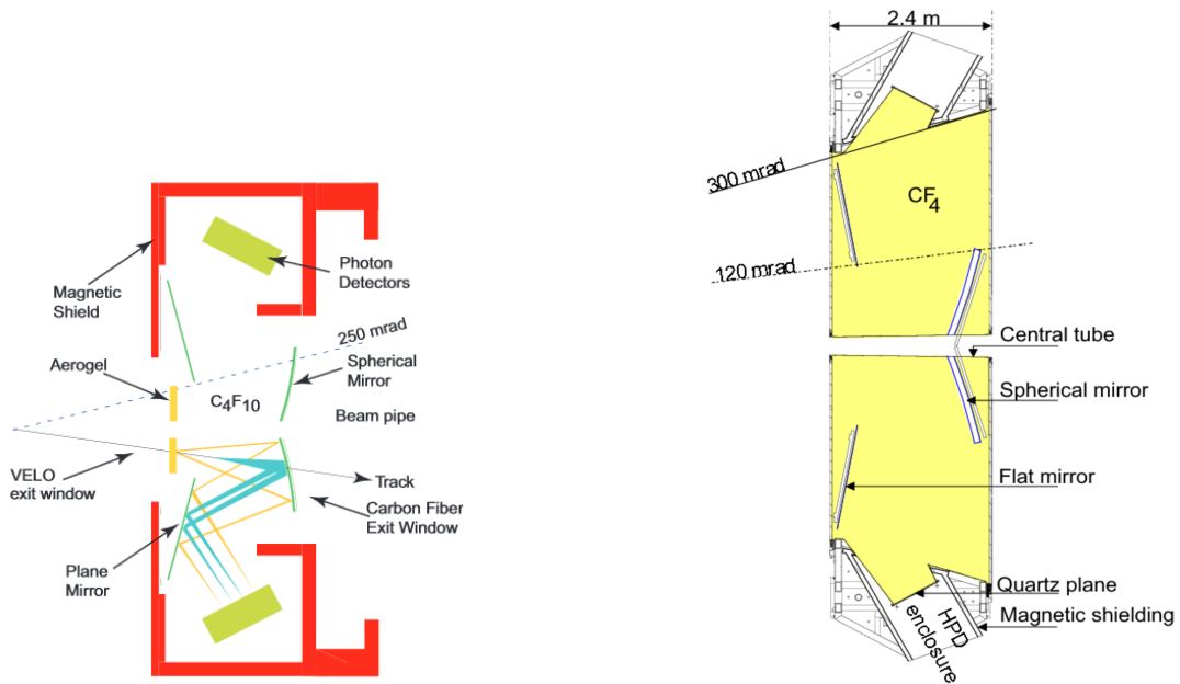
FIGURE 3.10: Layout of the RICH1 (left) and RICH2 (right).
