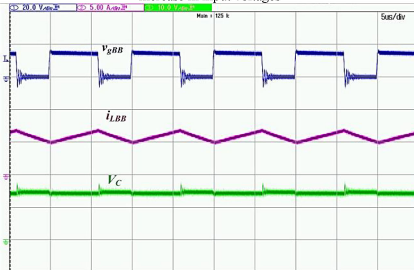
(c) Gate voltage of Q_{BB} , inductor current i_{LBB} and capacitor voltage V_C at 10% decrease in input voltages
