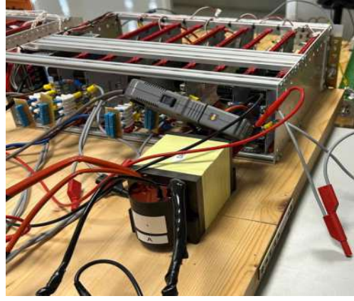
Fig. 5. Experimental setup of H-bridge utilized silicon carbide (SiC) MOSFETs.
