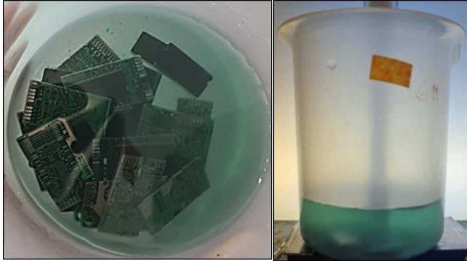
Figure 8.13 – Sample 3 treatment in an open beaker under room temperature and mechanical stirring, in the presence of H_2O_2 .
