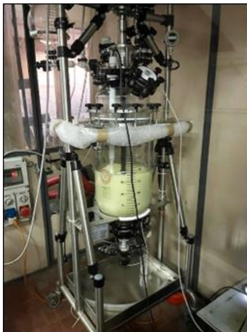
Figure 7.5 – Fermentation reactor (30 L working volume).
