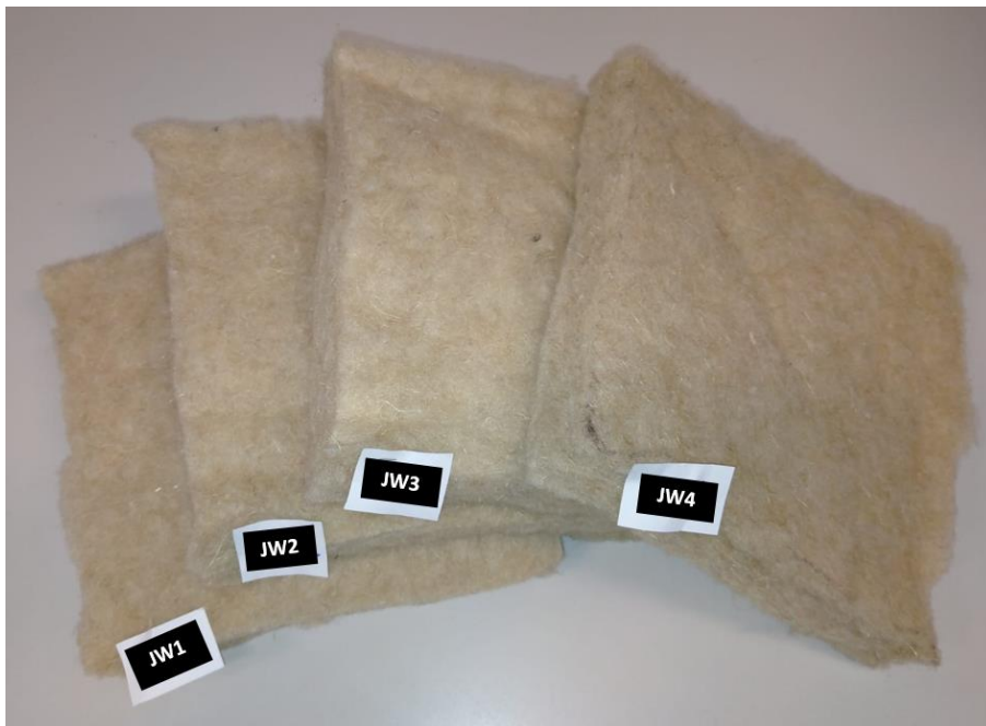
Figure 2 - Insulation panel made of recycled jute and wool fiber.
