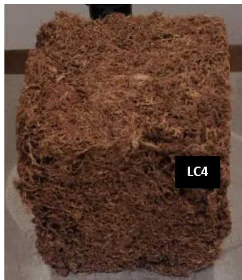
Figure 6. Insulation materials: Loofah fiber and clay used as binding material
