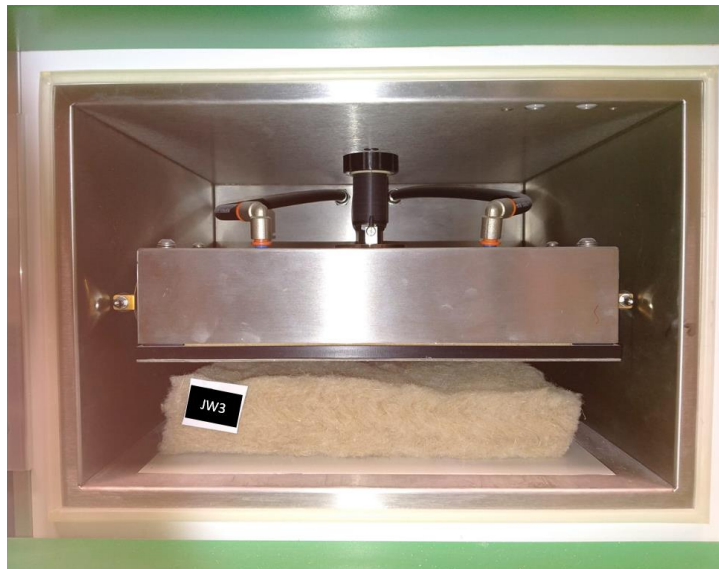
279 280 Figure 8 - Sample JW3 with 250 \times 250 \text{ mm}^2 inside the TAURUS measuring chamber.
