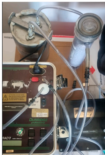
Figure 1. A photo of the experimental set-up for the radon exhalation assessment.
