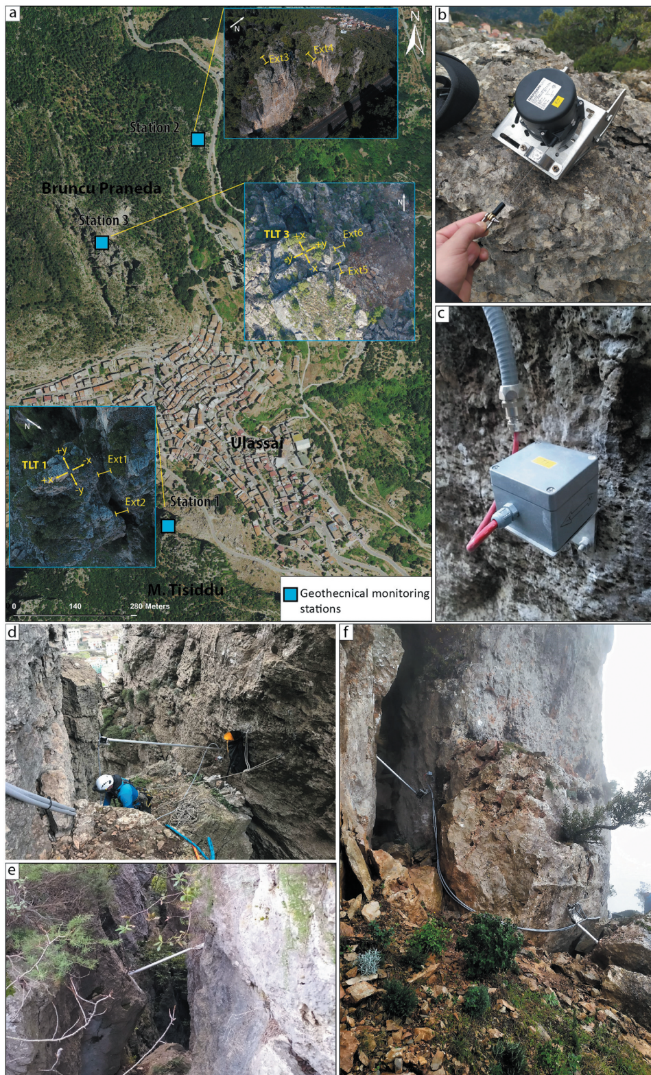
Figure 6. a) Geotechnical station instrumentations location. b) Extensimeter GEFRAN GSF1800 d c) Tiltmeter T1 MEMS Earth System (from Demurtas V. et al 2021); d) Extensimeter Ext 1; e) Extensimeter Ext 3; f) Sensor installed in the station 3.
