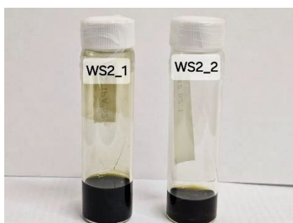
Figure A.2 Image of WS 2 dispersions after a completed exfoliation in IPA followed by centrifugation.
