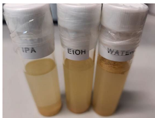
Figure A.1 Image of PhCN dispersions after 8h sonication in different solvents for liquid phase exfoliation
