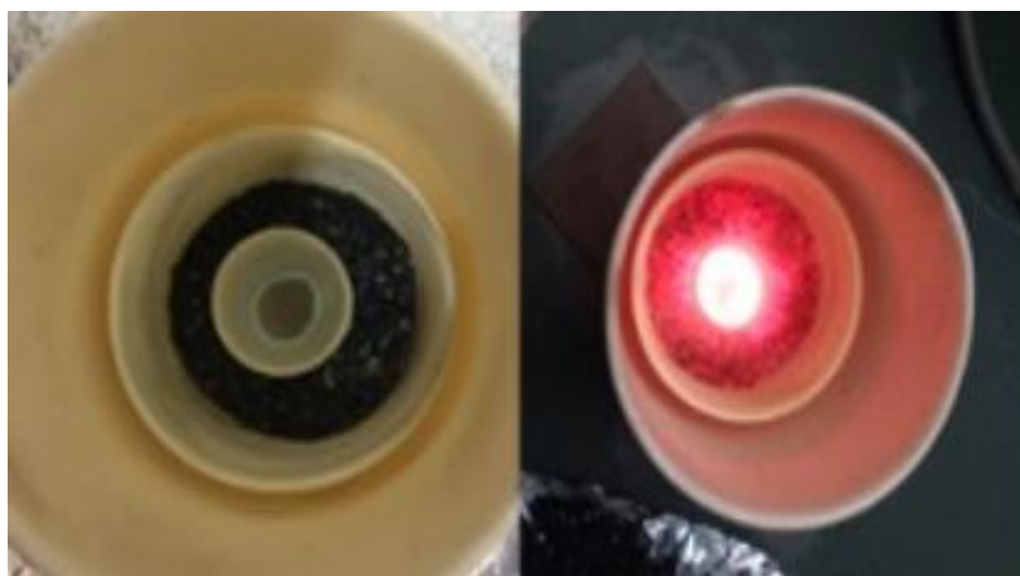
Figure 15. View of the Microwave assisted synthesis (MAS), on the left: the sample after the synthesis, on the right, during the synthesis.
