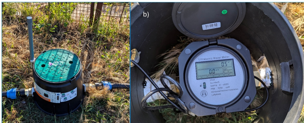
Figure 3.21: (a) Installation of the LoRaWAN ultrasonic water meter within a protective housing connected to the irrigation line (b) An internal view of the ultrasonic flow sensor and the display unit with LoRaWAN communication module.
