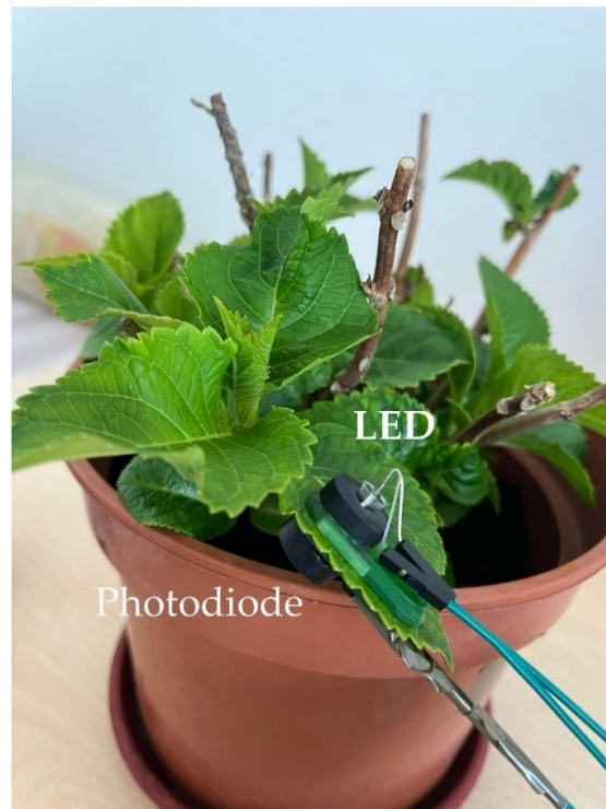
Figure 3.4: Photograph of the corresponding sensor prototype attached to a plant leaf, where the LED and photodiode are mounted on opposite faces of a custom 3D-printed clip, designed with embedded magnets for securing attachment to the leaf.
