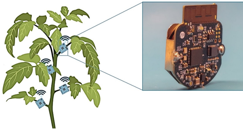
Figure 3.7: Overview of the petiole sensor module developed by the DRAMCO group at KU Leuven.
