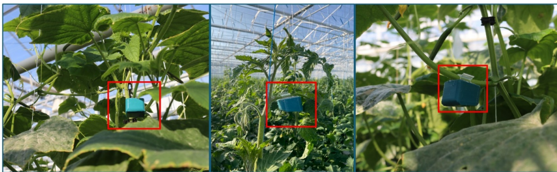
Figure 3.12: Deployment of IMU-based sensor modules in greenhouses under different environmental conditions.
