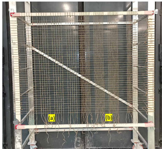
Figure 2. Jute net fabrication (a) 2.5 cm × 2.5 cm and (b) 2.5 cm × 1.25 cm mesh configurations.
