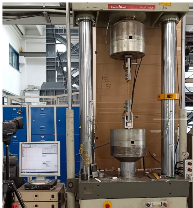
Figure 6. Schenck universal machine used for tensile strength tests.
