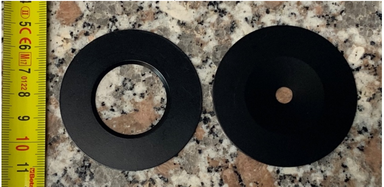
Fig. 5. The 25.4 mm diameter and the 4 mm diameter target masks used in this study.
