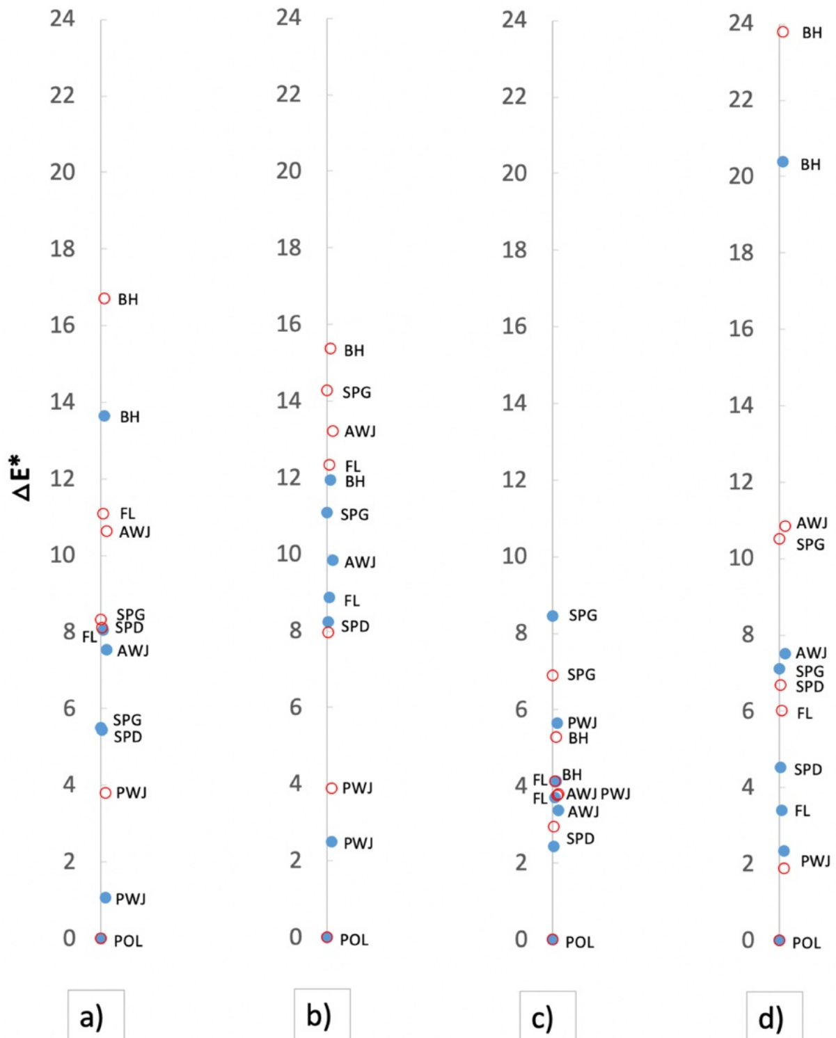
Fig. 9. Total colour differences ( \Delta E^* ) in Ghiandone (a), K-feldspar (b), plagioclase (c) and quartz (d) for each surface finishings.
