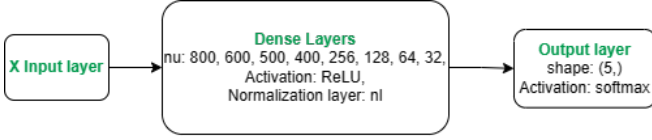
Fig. 2. The architecture of FC-DNN1. The input dataset X is D_1 for PV_1 , D_2 for PV_2 , and D for FV .
