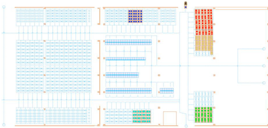
Figure 1 – Layout and location of pallets inside the bay
