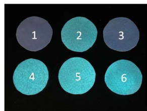
Figure 10. Fluorescence photographs (under UV 365 light) of test papers containing the [Zn L2 ] 2+ complex upon addition of the different analytes: 1 = L2 , 2 = [Zn L2 ] 2+ , 3 = [Zn L2 ] 2+ + H 3 PMG, 4 = [Zn L2 ] 2+ + H 2 GLU, 5 = [Zn L2 ] 2+ + H 2 AMPA, 6 = [Zn L2 ] 2+ + CaHPO 4 .
