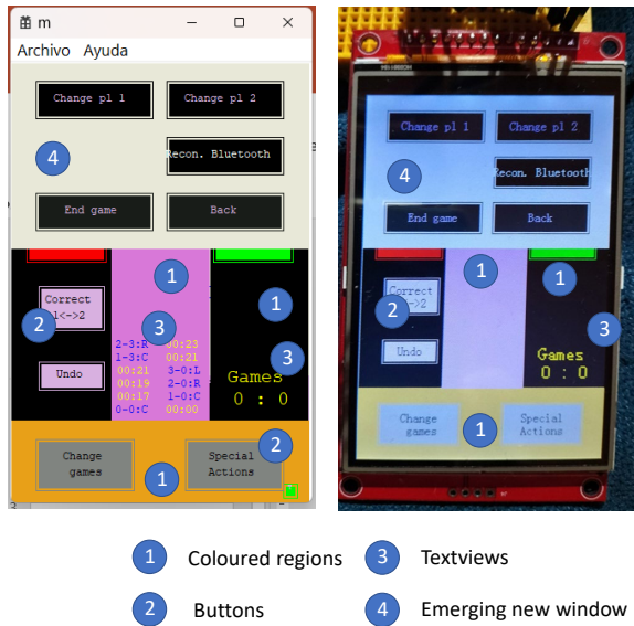
Fig. 5. A window of the user defined GUI with an emerging new window with buttons.
