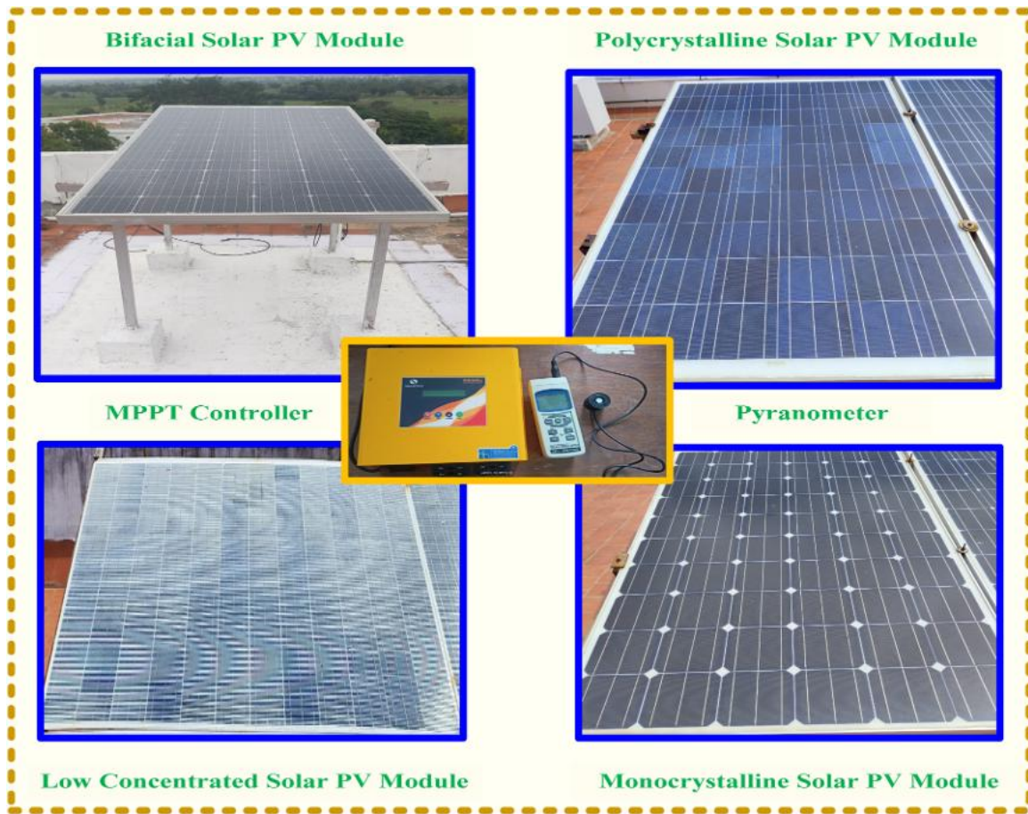
FIGURE 2 | Experimental setup of PPVM, MPVM, LPVM, and BPVM.
