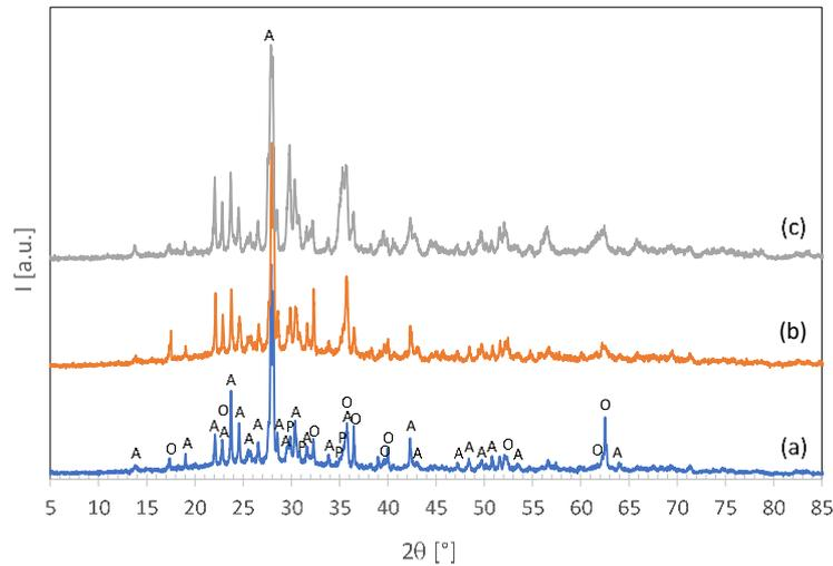
**Figure 1.** XRD patterns of (a) starting Lunar regolith simulant and corresponding SPS products obtained at (b)  $T_D= 700^\circ\text{C}$  and (c)  $T_D= 900^\circ\text{C}$ . A = Sodium Calcium Aluminum Silicate Anorthite, sodian disordered; O = Magnesium Iron Silicate Olivine; P = Calcium Magnesium Aluminum Titanium Silicate Clinopyroxene.
