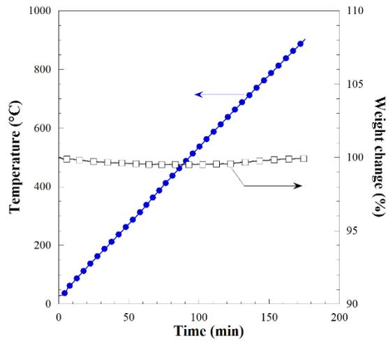
**Figure 3.** Weight change (%) of JSC-1A regolith during TGA experiment under dynamic conditions.
