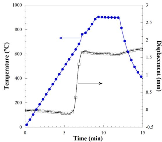
**Figure 4.** Sample displacement and corresponding temperature time profiles recorded during the consolidation by SPS of Lunar regolith powders for the case of  $T_D=900^\circ\text{C}$ .
