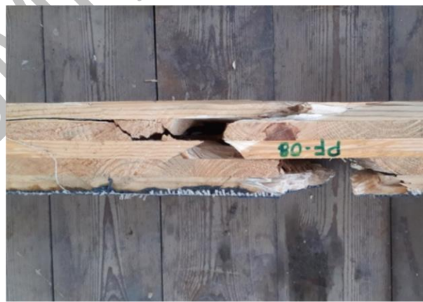
Fig. 11. Rupture mechanism of the single layer strengthened 100-PF-08CLT specimen. (a) Global brittle bending failure, (b) Local flexural cracks.
