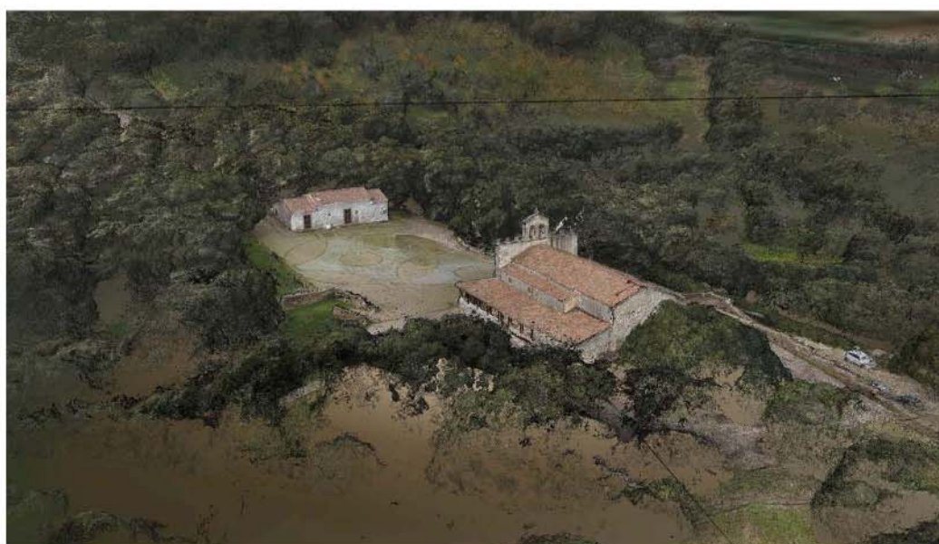
Fig. 5. Dense point cloud created from video sequence frames with the aim of acquiring a broader context and designing the survey. Elaborations by Nicola Paba, scientific coordination Andrea Pirinu.
