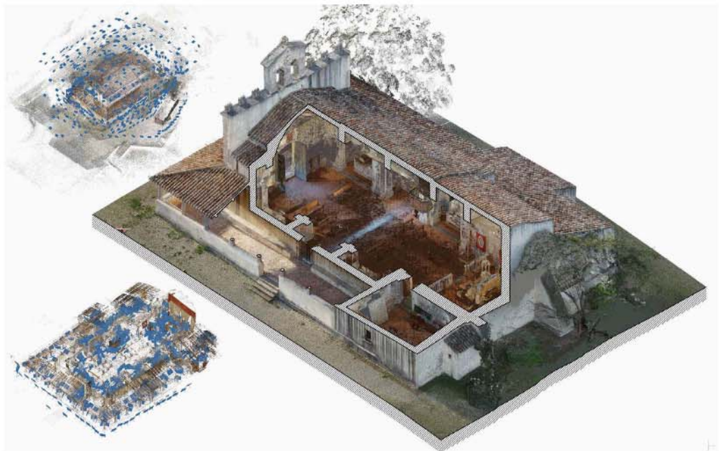
Fig. 7. Axonometric view of the point clouds (external and internal) and restitution of the axonometric cross-section obtained starting from their alignment. Elaboration by Nicola Paba, scientific coordination Andrea Pinnu.
