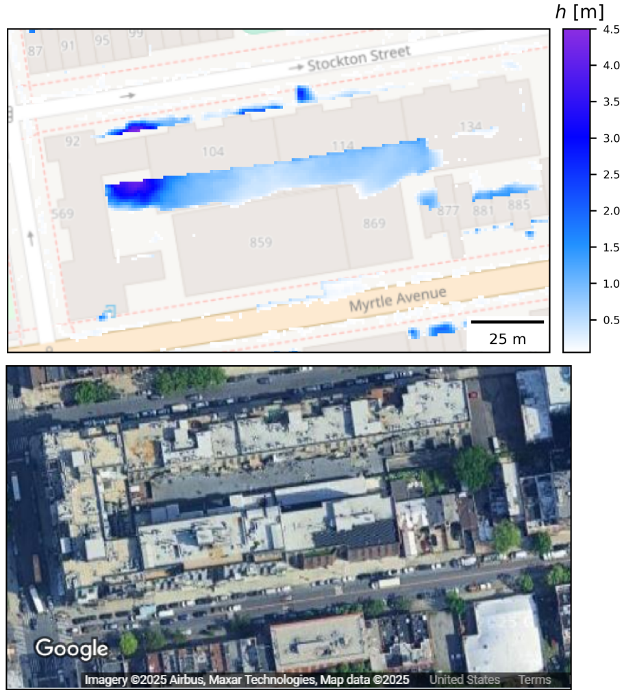
Figure C.7: Top panel: high water depth simulated with the Out-SW approach in the terrain depression in the CB shown by rectangle C7 in Figure C.1; the base map is from OpenStreetMap. Bottom panel: aerial view of the buildings obtained from Google Satellite and Airbus, Maxar Technologies imagery, which does not seem to indicate the presence of depression. These might be due to inaccuracies in the DTM.
