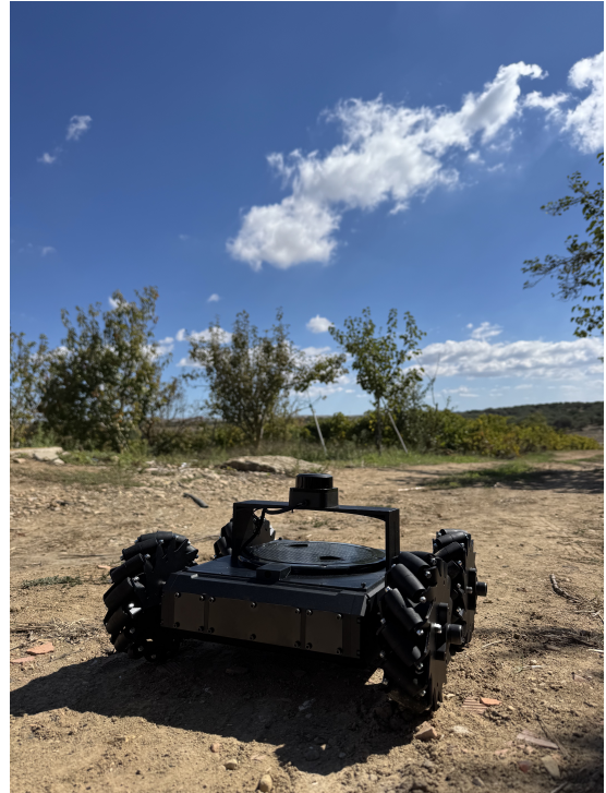
(b) Prototype UGV used in AGROS
