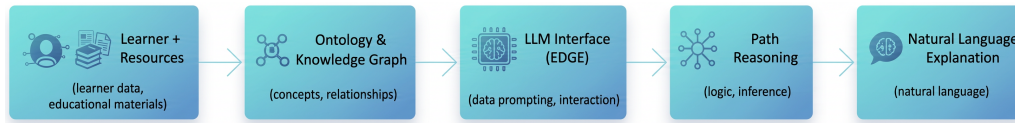
Fig. 1.1: Integrated pipeline for explainable lifelong learning. Learner data and educational resources are structured through ontology-driven knowledge graphs, accessed through an LLM-based interface (EDGE), processed through path reasoning for explainable recommendations, and finally transformed into natural language explanations to support user understanding and decision-making
