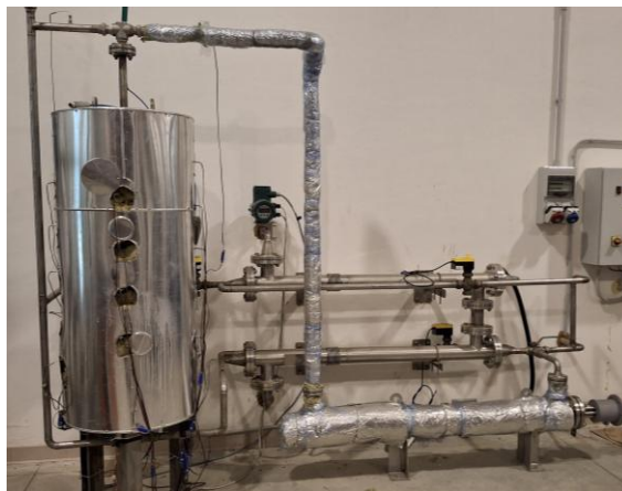
Figure 1. Test rig with thermal energy storage system.
