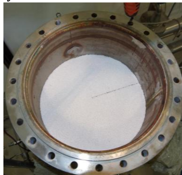
Figure 2. Cylindrical tank filled with alumina balls
