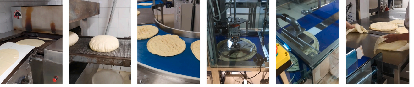
Fig. 1. Pictures of Carasau production process showing the steps of baking in the oven, cooling/drying over the conveyor belt, and automated separation.
