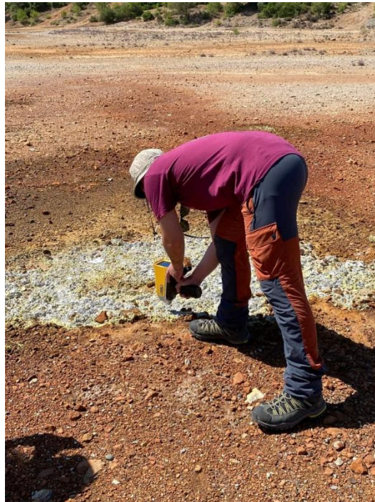
Figure 21. Field use of portable X-ray fluorescence (p-XRF) for the geochemical screening of secondary mineral patinas in flotation tailings at the Campo Pisano mine.
