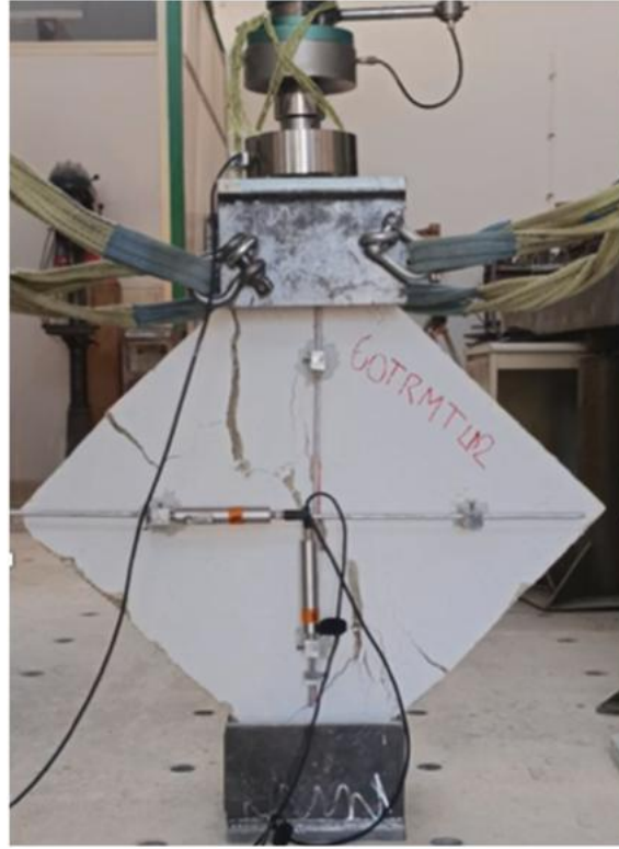
Fig. 27. Diagonal tension (shear) test: 60TRMTLD2 after the test.
