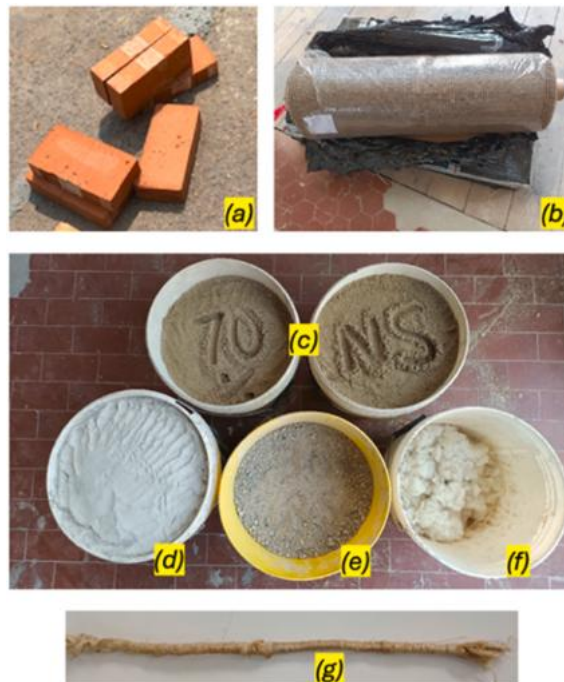
Fig. 2. (a) Clay bricks, (b) flax net, (c) natural sand, (d) NHL(5F) natural hydraulic lime, (e) recycled sand, (f) chopped sheep wool, and (g) jute fiber diaton.
