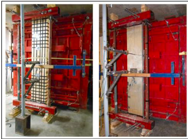
Fig. 15. CLT specimens strengthened with (a) steel straps and (b) GFRP [152].
