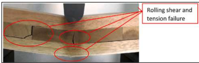
Fig. 3. Rolling shear failure [108].
