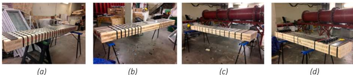
Fig. 17. CLT retrofitted with man-made fibers, with various configurations: (a) Specimen 4, (b) Specimen 5, (c) Specimen 6, and Specimen 7 [152].
