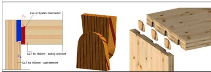
Fig. 7. Wood-wood system connections [117].
