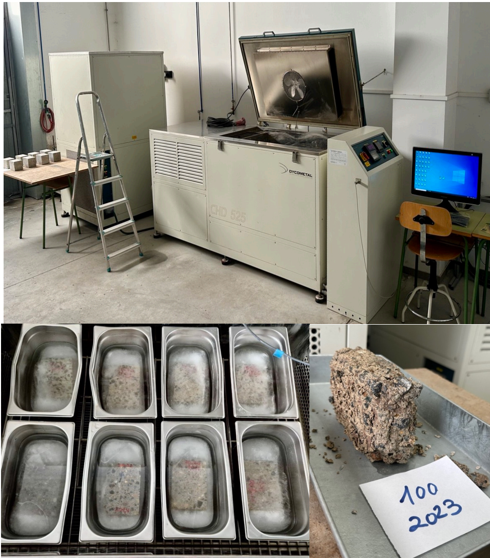
Figure 24. Freeze-thaw resistance test.
