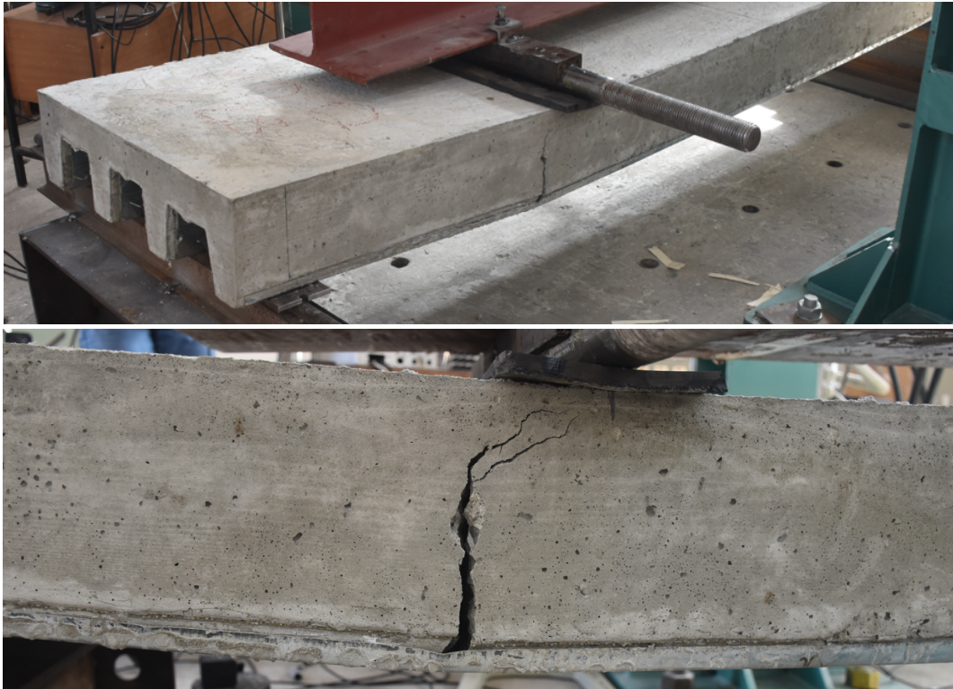
Figure 37. Flexural crack at the end of the test.
