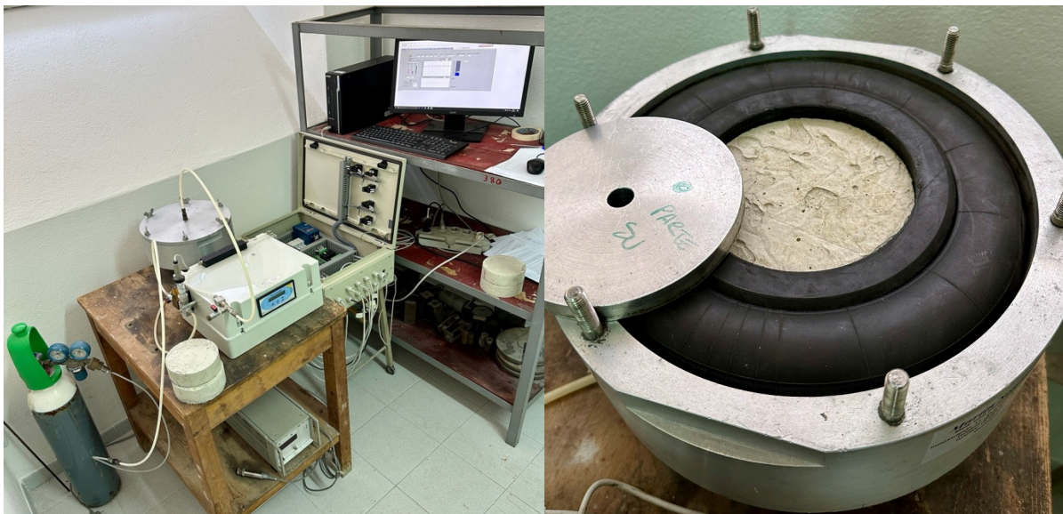
Figure 18. Oxygen permeability test.
