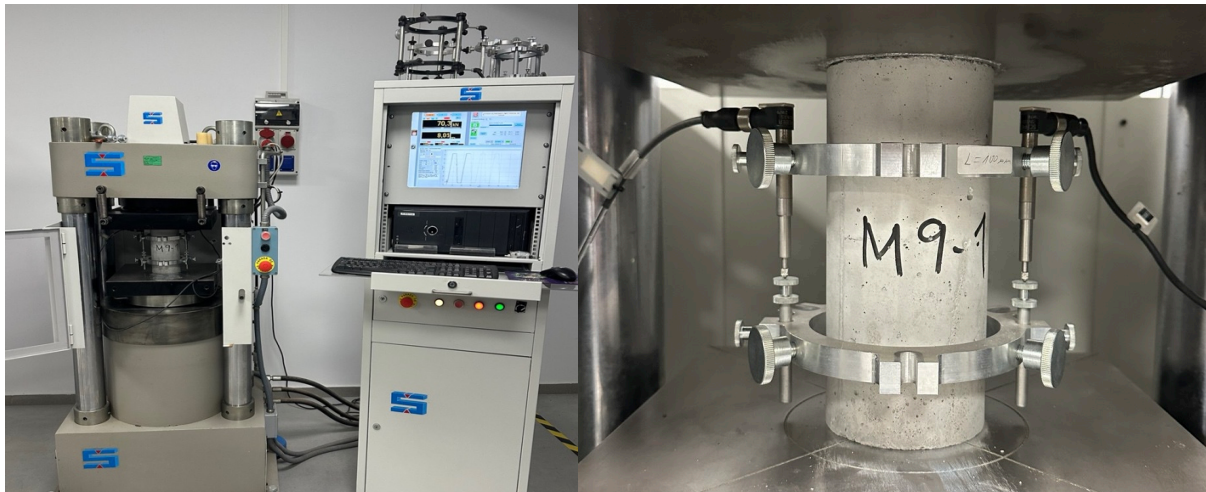
Figure 16. Modulus of Elasticity test.
