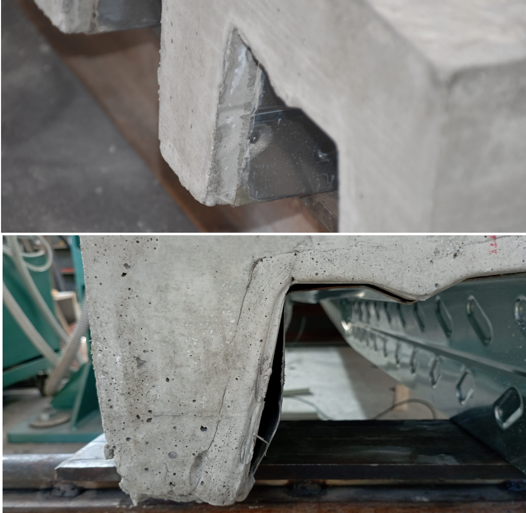
Figure 36. Typical relative displacements of the steel sheet with respect the concrete during the test.
