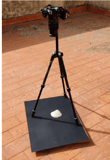
Fig. 4 Shooting setting for the seashell dataset. The whole system is placed upon a rotating platform.
