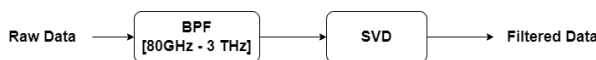
Fig. 5. Signal Filtering Procedure: Step 1 - Band Pass Filter (BPF); Step 2 – Filtering procedure based on the data matrix Singular Value Decomposition (SVD).
