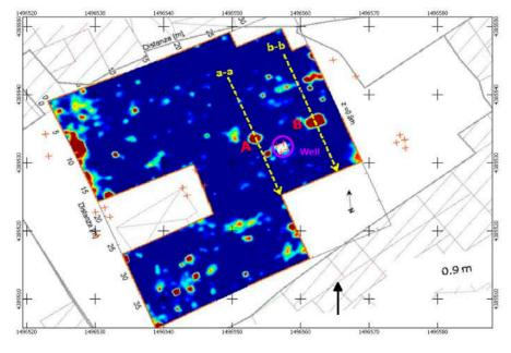
**Figure 12.** Radargrams crossing the two big anomalies of the GPR map at a 90-cm depth: (a) The GPR map; (b) Profile a-a; (c) Profile b-b.
