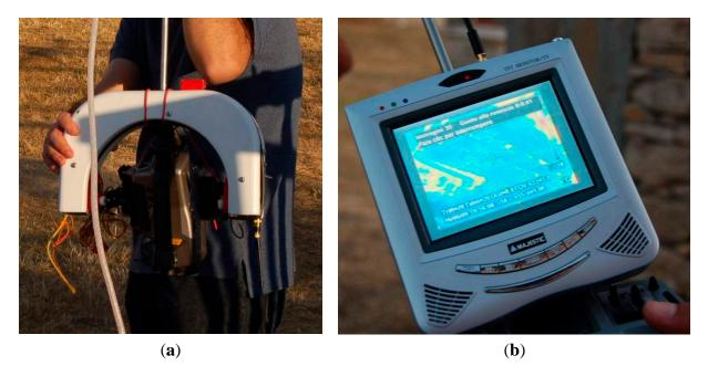
The acquisition instrumentation was hung by means of the fastening system mentioned above to a balloon, inflated with about 15 cubic meters of helium, anchored to the ground on a three-ballast fixture and with an additional fourth security cable that was slack (Figure 5). The height of the camera was about 50 m, and it was located to ensure the coverage of the northern area, the range of the driveway, the first of two wells and part of the excavated necropolis.
