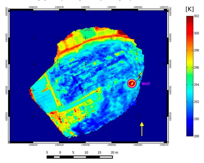
**Figure 6.** The thermal map of apparent intercept temperature (in Kelvin degrees), resulting from the merging of many thermograms and processing temperature over time.
