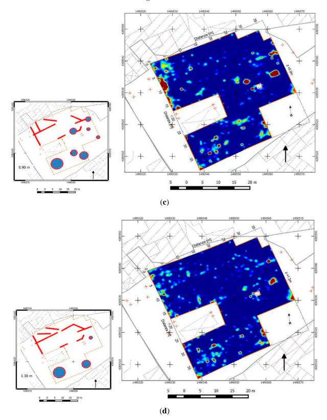
The GPR acquisition window was 256 ns with 1024 samples per scan. The acquisition profile was equally spaced 0.50 m in two orthogonal directions for a total length of 4.045 km.
