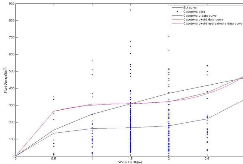
Figure 3. EU-JRC Residential use depth-damage curve and Capoterra collected damage data
