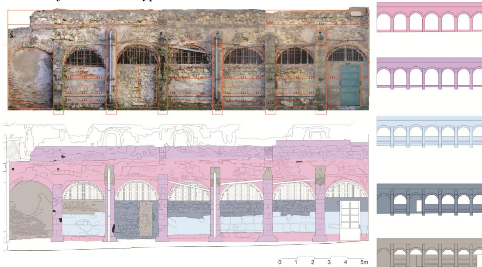
Figure 4. The West Facade: Stratigraphic Analysis of the Structures, Dating and Transformations Hypothesis
