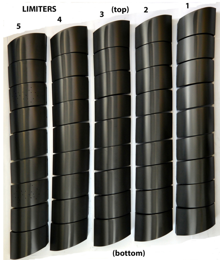
Figure 9. The five limiters from W7-X OP1.1, laid out in the laboratory after the run. Dual erosion/deposition stripes are noteworthy, and are remarkably similar on limiters 2–5, but differ strongly on the middle tiles of limiter 1 where the stripes fade away. There is a small top/bottom asymmetry in the stripe pattern on all five limiters. (The golden hue on some tiles is real, and is an interference film effect which is strongly dependent on the camera viewing angle).
