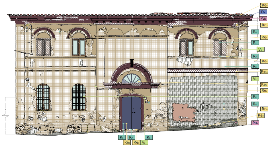
Fig. 6. Photogrammetric survey, analysis of materials, decay and conservative restoration of the facade (edit F. Meloni)
