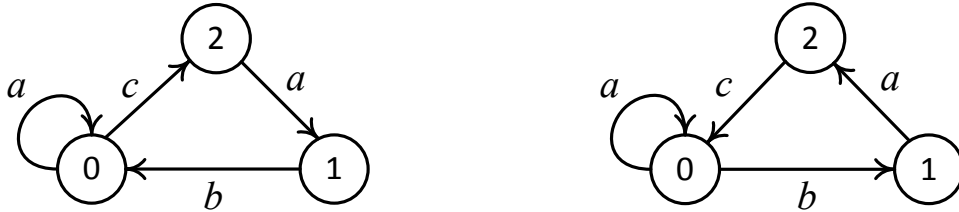
Fig. 2.3 DFA without specifying the initial state. Fig. 2.4 Reverse automaton of the DFA in Fig. 2.3.
