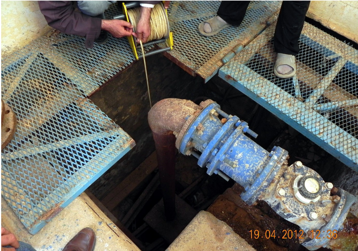
Fig. 3.4 Piezometric level measurements during WADIS-MAR survey (Photograph courtesy of Prof. G. Ghiglieri).
