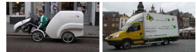
Figure 3.25. Electronic tricycle and natural gas truck used to make the deliveries
