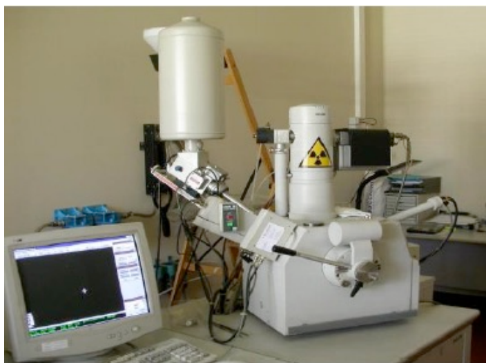
Fig. 3 Scanning Electron Microscopy (SEM) equipped with Energy Dispersive X-Ray (EDX) detector (Zeiss, Germany).
