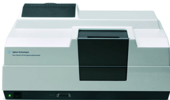
Fig. 4 UV spectrophotometer (Agilent Technologies, Cary Series Spectrophotometer).
