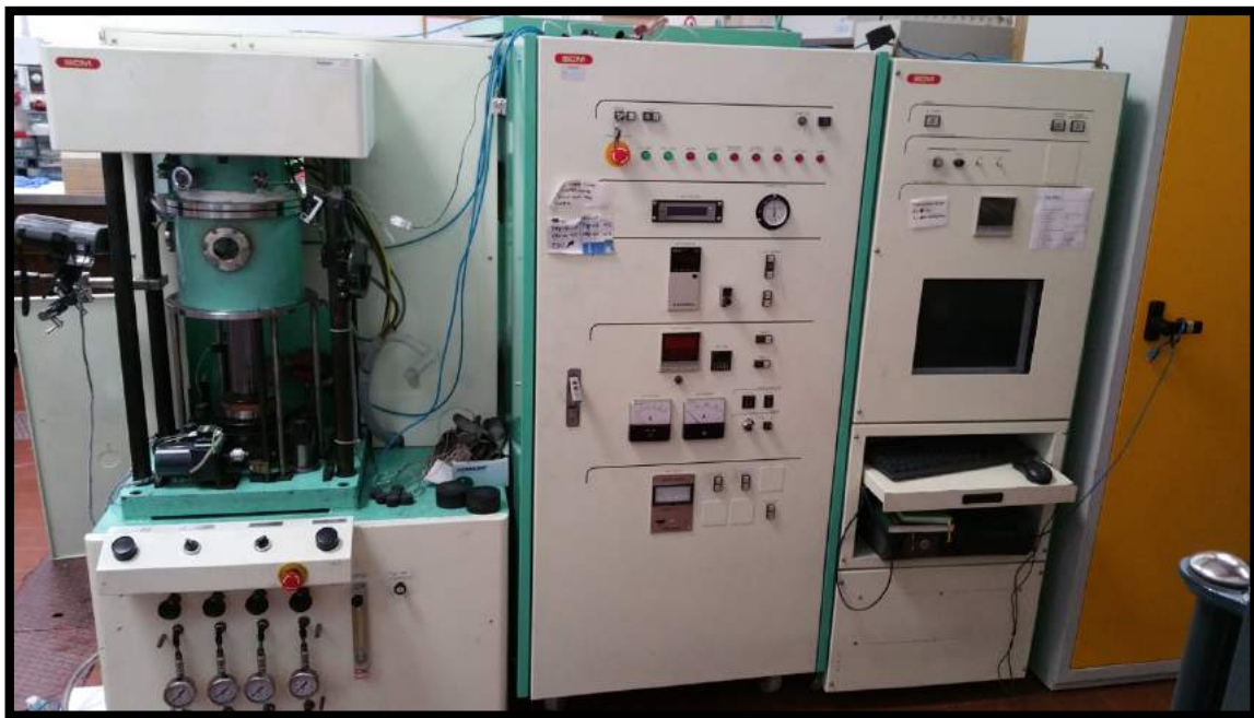
Figure 28. Spark Plasma Sintering apparatus (mod. 515S) used in this work.
