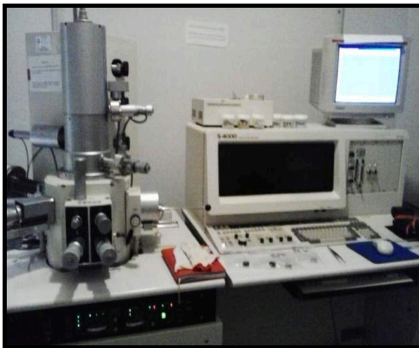
Figure 26. High resolution Scanning electron microscopy equipment (mod. Hitachi S4000).
