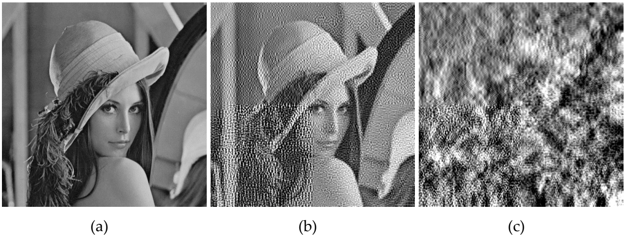
Figure 20 - Original "Lena" 512x512, 8bpp (a), "Lena" transmitted for SNR = 5dB, with the proposed modified 64-APSK 4+12+20+28 mapping (b), and conventional 64-APSK with CCSDS mapping (c).
