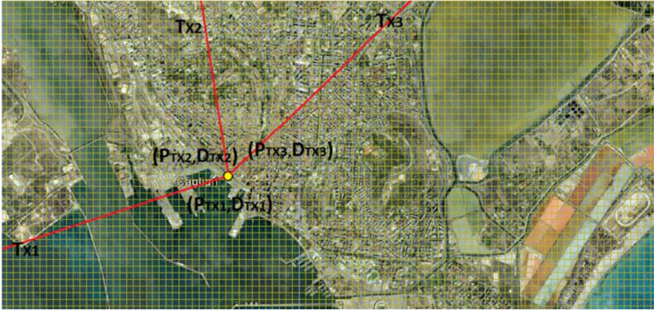
Figure 3 - Example of network simulation model: a yellow dot generic receiver contains information represented by three couples of power received and relative delay by three TXs
