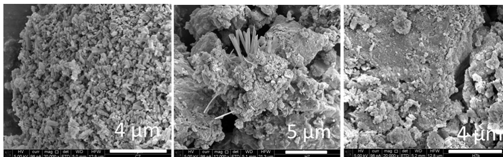
Figure 4.16. SEM images of compound (2 \cdot \mathbf{L1})_{\infty} : micro-crystals from conventional synthesis (left), NG sample after 40 minutes grinding (middle), LAG sample after 20 minutes grinding (right). Magnifications are reported in the bottom of the micrograph (bar= 4 \mu\text{m} (conventional and LAG sample) bar= 5 \mu\text{m} (NG sample)).
