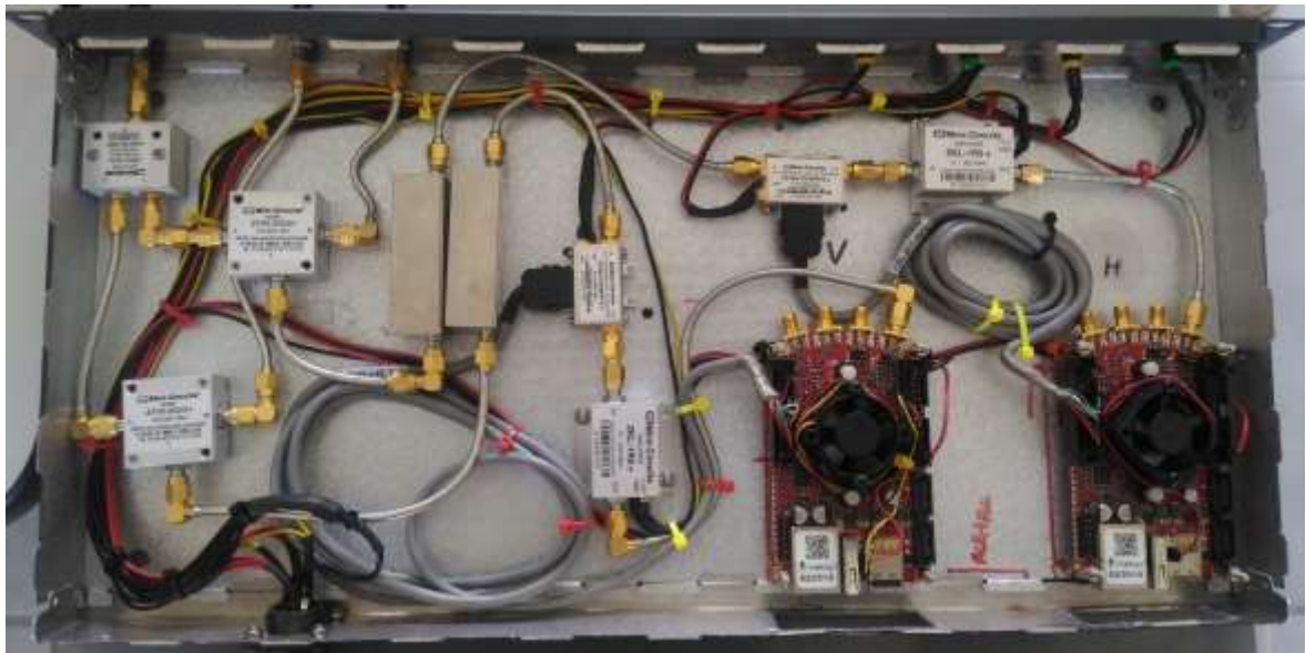
Fig. 6.15. Picture of the down-conversion and back-end section of the new receiving channel.
