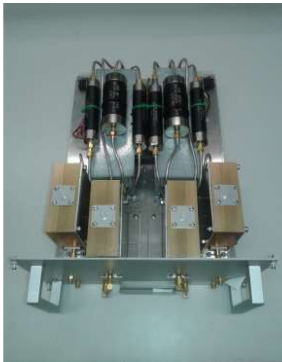
Fig. 6.6. Picture of the 16 MHz bandwidth tubular BPFs at 410 MHz (the larger ones) mounted inside the filter selector block of the P-band receiver.
